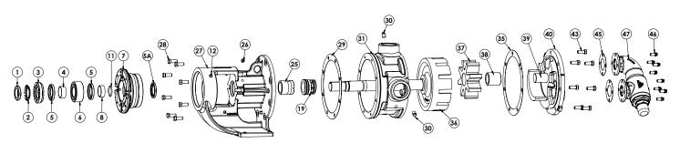
NOTE: Kit may not apply to all models of these pumps. Contact your Viking Pump distributor with pump serial number for correct kit part numbers for that pump. Both a Seal Kit & Rebuild Kit are needed to completely rebuild the pump. Additional non-kit parts, such as Rotor and Shaft Assembly, may also be required, depending on wear.
