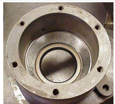
Figure 13, Inner bearing race installed
