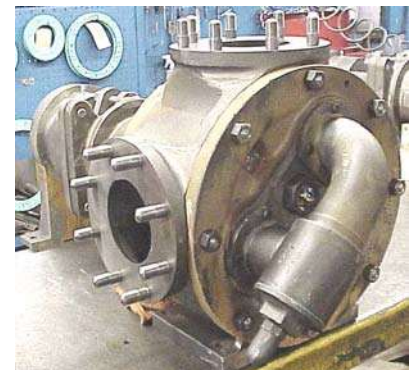
Figure 2, Standard head and relief valve orientation.
