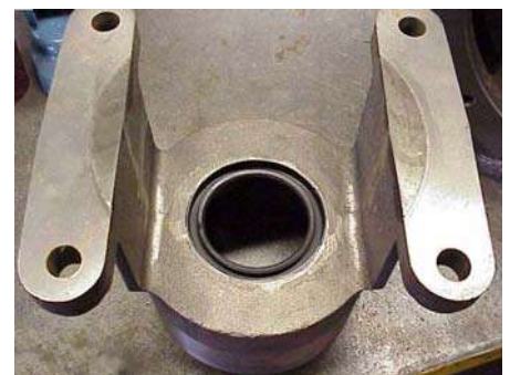
Figure 12, Inner lip seal orientation
