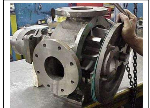
Figure 18 Installing the head
