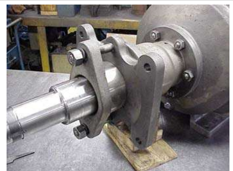
Figure 11, Packing gland installed
