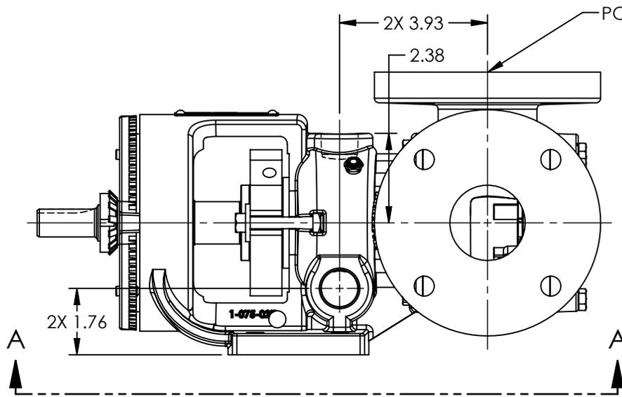
PORTS: 2X 2" FLANGES DRILLED AND TAPPED SUITABLE FOR USE WITH CLASS 125 ANSI FLANGES (1224A) CLASS 150 ANSI FLANGES (1227A)
