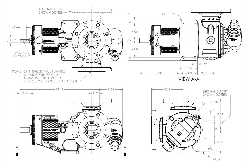
MODELS WITH OPTIONAL FLANGED PORTS: K123C, K4123C, K127C, K1127C, K4127C, KK123C, KK4123C, KK127C, KK1127C, KK4127C
