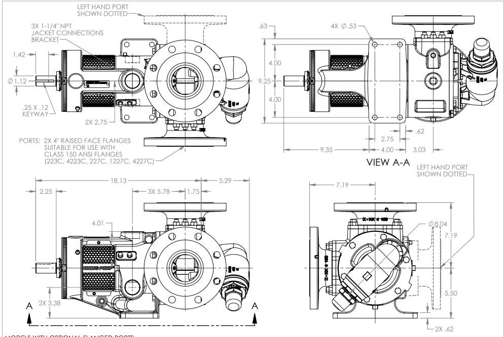
MODELS WITH OPTIONAL FLANGED PORTS: K223C, K4223C, K227C, K1227C, K4227C, KK223C, KK4223C, KK227C, KK1227C, KK4227C
