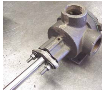
FIGURE 14: GLAND & FASTENERS INSTALLED
