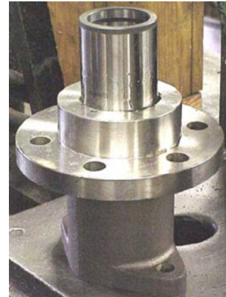
FIGURE 15: RBS BUSHING INSTALLATION
