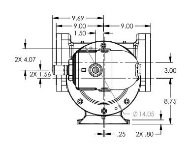
MODELS WITH OPTIONAL FLANGED PORTS: Q223C, Q4223C, Q227C, Q1227C, Q4227C
