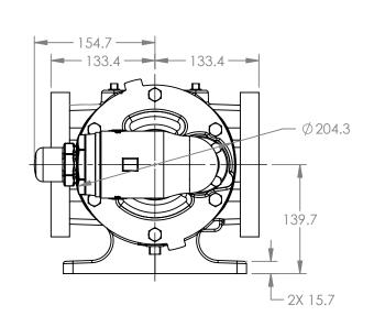
MODELS WITH OPTIONAL FLANGED PORTS: K123C, K4123C, K127C, K1127C, K4127C, KK123C, KK4123C, KK127C, KK1127C, KK4127C
