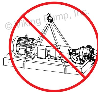
**NOTE: NEVER** lift the unit with slings unsecured under the base. The slings can slide, allowing the unit to tip and/or fall. Improper lifts can result in personal injury and/or damage to the unit.
