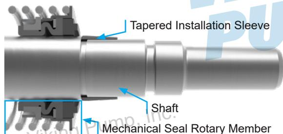
**NOTE:** Coat rotor shaft, tapered installation sleeve and inner diameter of mechanical seal with P-80® or equivalent before assembly.
