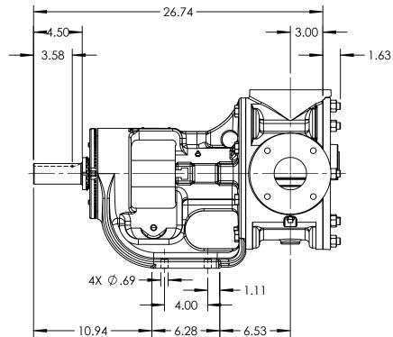
PORTS: 2X 3" FLANGES WITH STUDS AND NUTS (NOT SHOWN) SUITABLE FOR USE WITH **CLASS 125 ANSI FLANGES** (124A, 4124A, 4124B, 4624B) **CLASS 150 ANSI FLANGES** (126A, 4126A, 123A, 4123A, 127A, 4127A) 7.75 8.75 .80 4.12 4.12 - 10.00
