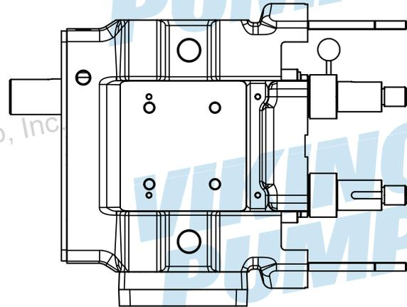
2. Drain oil, remove gear box cover and inspect gears for wear, backlash, and looseness. Retighten as needed.
