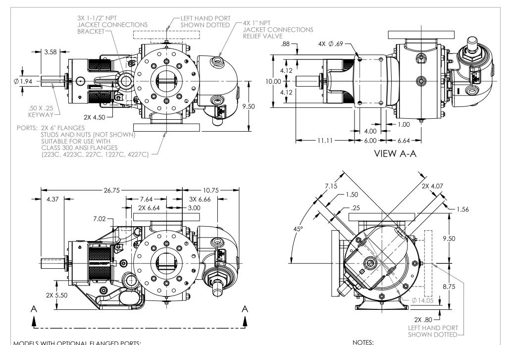
MODELS WITH OPTIONAL FLANGED PORTS: Q223C, Q4223C, Q227C, Q1227C, Q4227C
