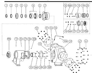
**NOTE:** Kit may not apply to all models of these pumps. Contact your Viking Pump distributor with pump serial number for correct kit part numbers for that pump. Both a Seal Kit and a Rebuild Kit are needed to completely rebuild the pump. Additional non-kit parts, such as Rotor and Shaft Assembly, may also be required, depending on wear.
