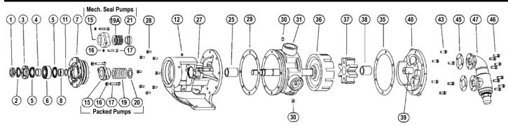
**NOTE:** Kit may not apply to all models of these pumps. Contact your Viking Pump distributor with pump serial number for correct kit part numbers for that pump. Both a Seal Kit and a Rebuild Kit are needed to completely rebuild the pump. Additional non-kit parts, such as Rotor and Shaft Assembly, may also be required, depending on wear.
