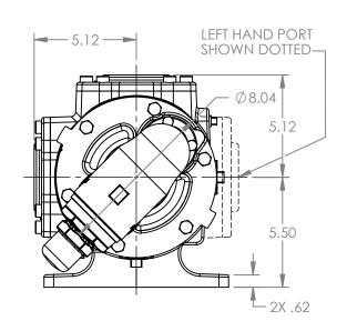
MODELS WITH OPTIONAL PORTS: K123C, K4123C, K127C, K1127C, K4127C, KK123C, KK4123C, KK127C, KK1127C, KK4127C
