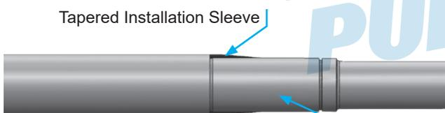
**NOTE:** Coat rotor shaft, tapered installation sleeve and inner diameter of mechanical seal with P-80® or equivalent before assembly.
