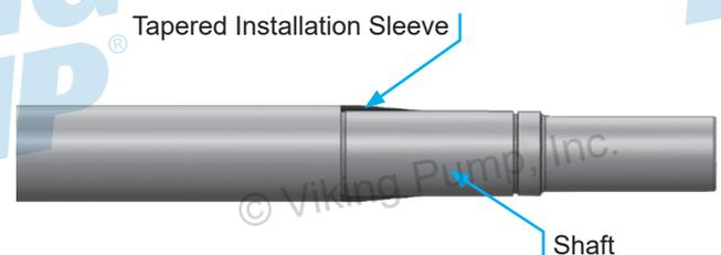
**NOTE:** Coat rotor shaft, tapered installation sleeve and inner diameter of mechanical seal with P-80® or equivalent before assembly.
