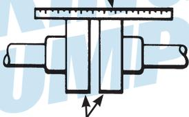
Check width between these surfaces with inside calipers to be certain the faces are equal distance apart and parallel.
