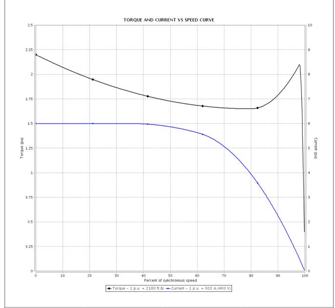
Performance : 460 V 60 Hz 6P Rated current : 603 A Moment of inertia (J) : 368 sq.ft.lb **LRC** : 6.0 Duty cycle : Cont.(S1) : 2180 ft.lb Insulation class : F Rated torque : 220 % Locked rotor torque Service factor : 1.15 Breakdown torque : 210 % Temperature rise : 80 K Rated speed : 1190 rpm
