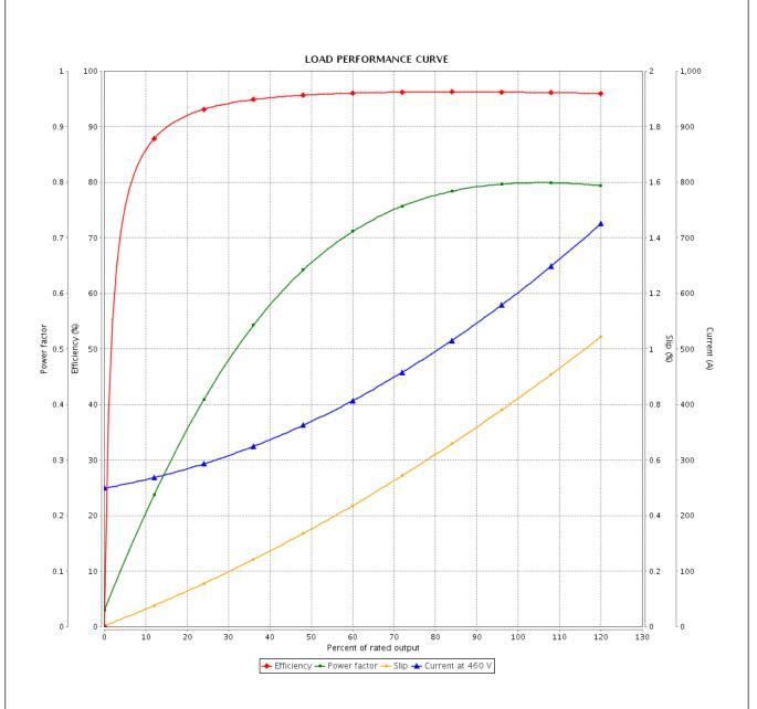
Performance : 460 V 60 Hz 6P : 603 A Moment of inertia (J) : 368 sq.ft.lb Rated current **LRC** : 6.0 Duty cycle : Cont.(S1) : 2180 ft.lb Insulation class : F Rated torque Locked rotor torque : 220 % Service factor : 1.15 Breakdown torque : 210 % Temperature rise : 80 K Rated speed : 1190 rpm
