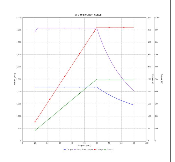
Performance : 460 V 60 Hz 6P Rated current : 603 A Moment of inertia (J) : 368 sq.ft.lb **LRC** : 6.0 Duty cycle : Cont.(S1) : 2180 ft.lb Rated torque Insulation class : F Locked rotor torque : 220 % Service factor : 1.15 Breakdown torque : 210 % Temperature rise : 80 K Rated speed : 1190 rpm
