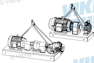
NOTE: Use two or more lifting slings around the pump and the motor when the base does not have lifting features.
