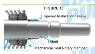
**NOTE:** Coat rotor shaft, tapered installation sleeve and inner diameter of mechanical seal with P-80® or equivalent before assembly.
