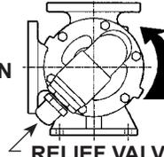
RELIEF VALVE ADJUSTING SCREW CAP
