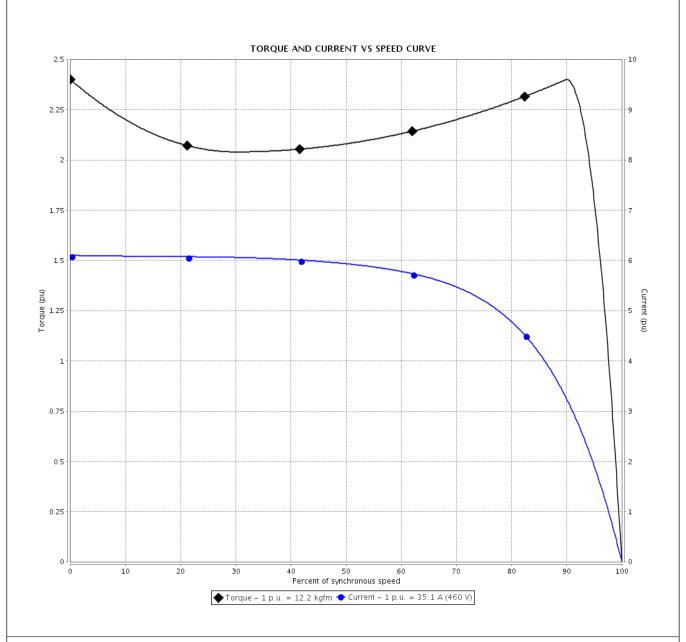
Performance : 208-230/460 V 60 Hz 4P Rated current : 77.6-70.2/35.1 A Moment of inertia (J) : 0.2467 kgm<sup>2</sup> **LRC** Duty cycle : Cont.(S1) : F : 12.2 kgfm Insulation class Rated torque : 240 % Service factor Locked rotor torque : 1.25 Breakdown torque : 240 % Temperature rise : 80 K Rated speed : 1765 rpm Design : B
