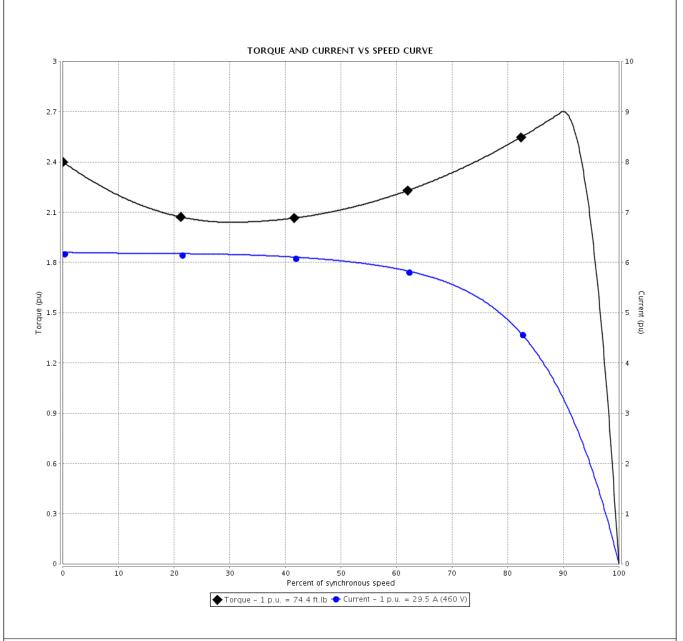
: 230/460 V 60 Hz 4P Performance Rated current : 59.0/29.5 A Moment of inertia (J) : 5.11 sq.ft.lb **LRC** : 6.2 Duty cycle : Cont.(S1) : 74.4 ft.lb Insulation class Rated torque : F : 240 % Service factor Locked rotor torque : 1.25 Breakdown torque : 270 % Temperature rise : 80 K Rated speed : 1765 rpm Design : B
