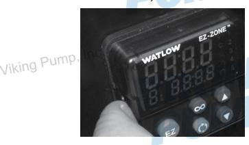
2. Once the sides are released grab the unit above and below the face with two hands and pull the unit out.
