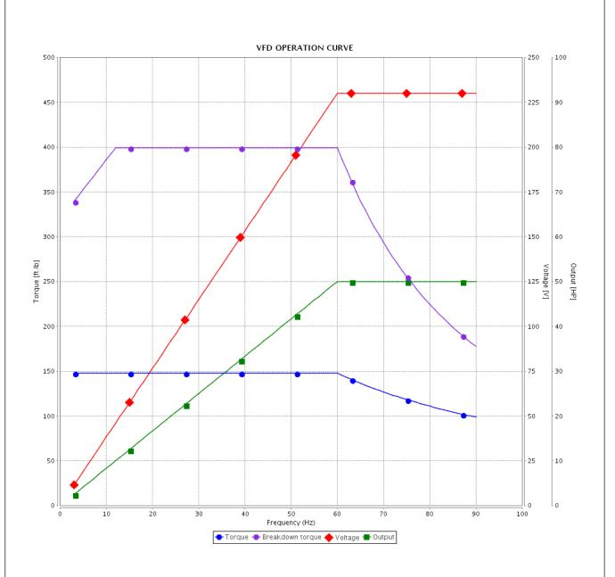
Performance : 208-230/460 V 60 Hz 4P : 131-118/59.2 A Rated current Moment of inertia (J) : 9.16 sq.ft.lb **LRC** Duty cycle : Cont.(S1) : 6.2 Insulation class : 148 ft.lb : F Rated torque Locked rotor torque : 229 % Service factor : 1.25 Breakdown torque : 270 % Temperature rise : 80 K Rated speed : 1775 rpm Design : B Rev. Performed Checked **Changes Summary** Date Performed by Checked by Revision Page
