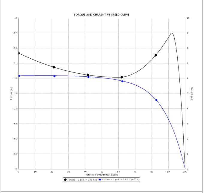
Performance : 208-230/460 V 60 Hz 4P Rated current : 131-118/59.2 A Moment of inertia (J) : 9.16 sq.ft.lb **LRC** : 6.2 Duty cycle : Cont.(S1) Insulation class Rated torque : 148 ft.lb : F Service factor Locked rotor torque : 229 % : 1.25 Breakdown torque : 270 % Temperature rise : 80 K Rated speed : 1775 rpm Design : B
