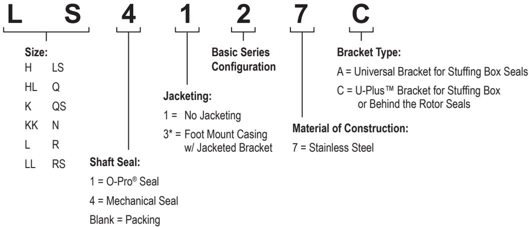
\* Note: Only the N through RS sizes are foot mount casing with jacketed bracket.
