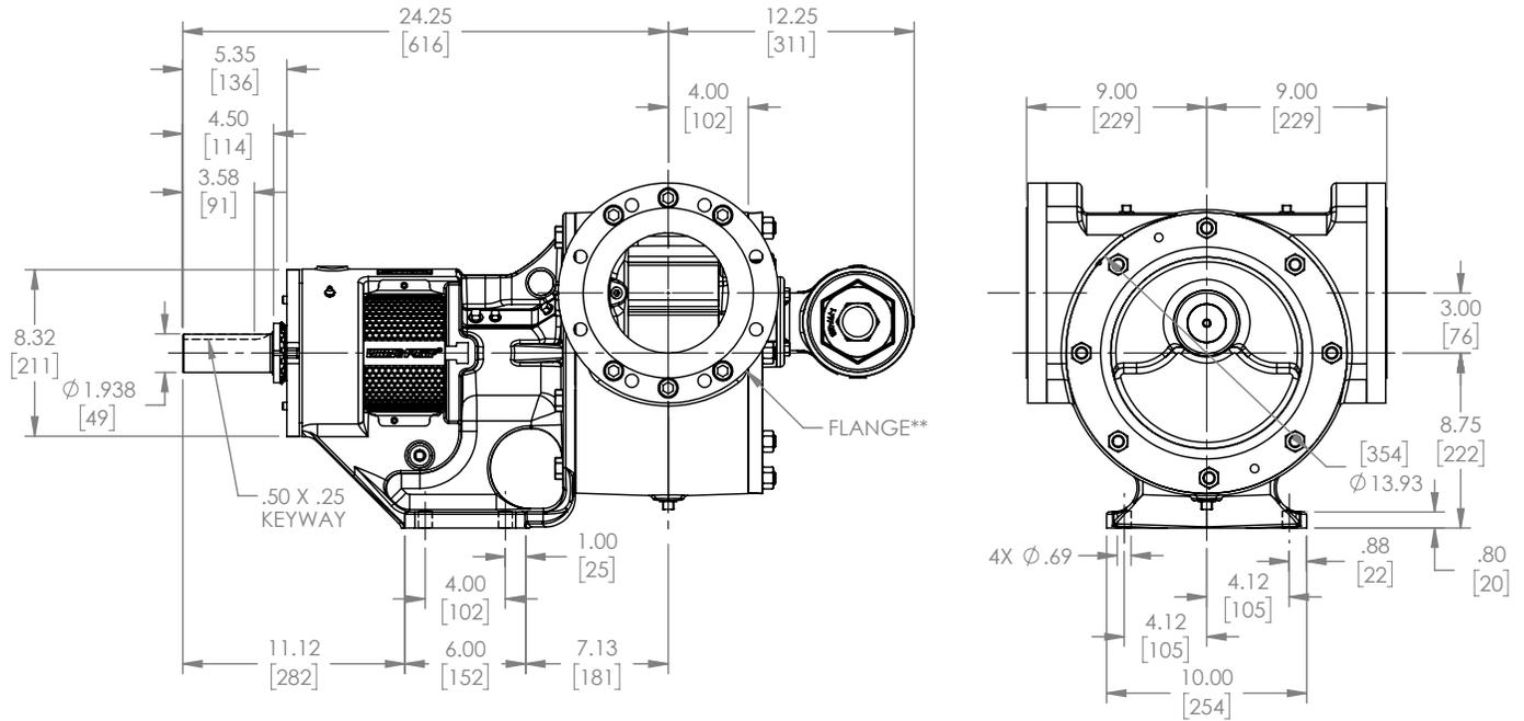
\*\* 127C Series™ / 1127C Series™ / 4127C Series™ ports suitable for use with Class 150 ANSI stainless steel companion flanges or flanged fittings. Ports are tapped for installation of studs..
