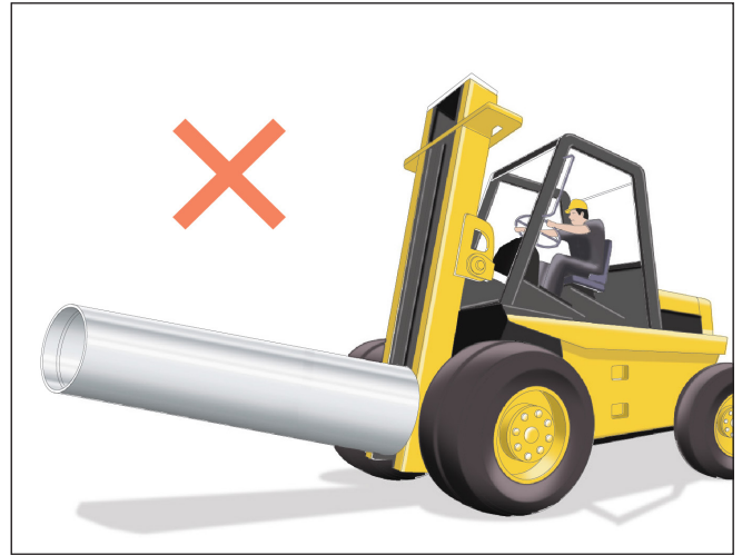
Figure 9 – Incorrect handling – do not lift through centre of pipe
