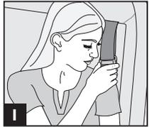
10. Make sure the lap-shoulder belt is snug and lies flat against the passenger. There should be no twisting of the webbing. **J**
