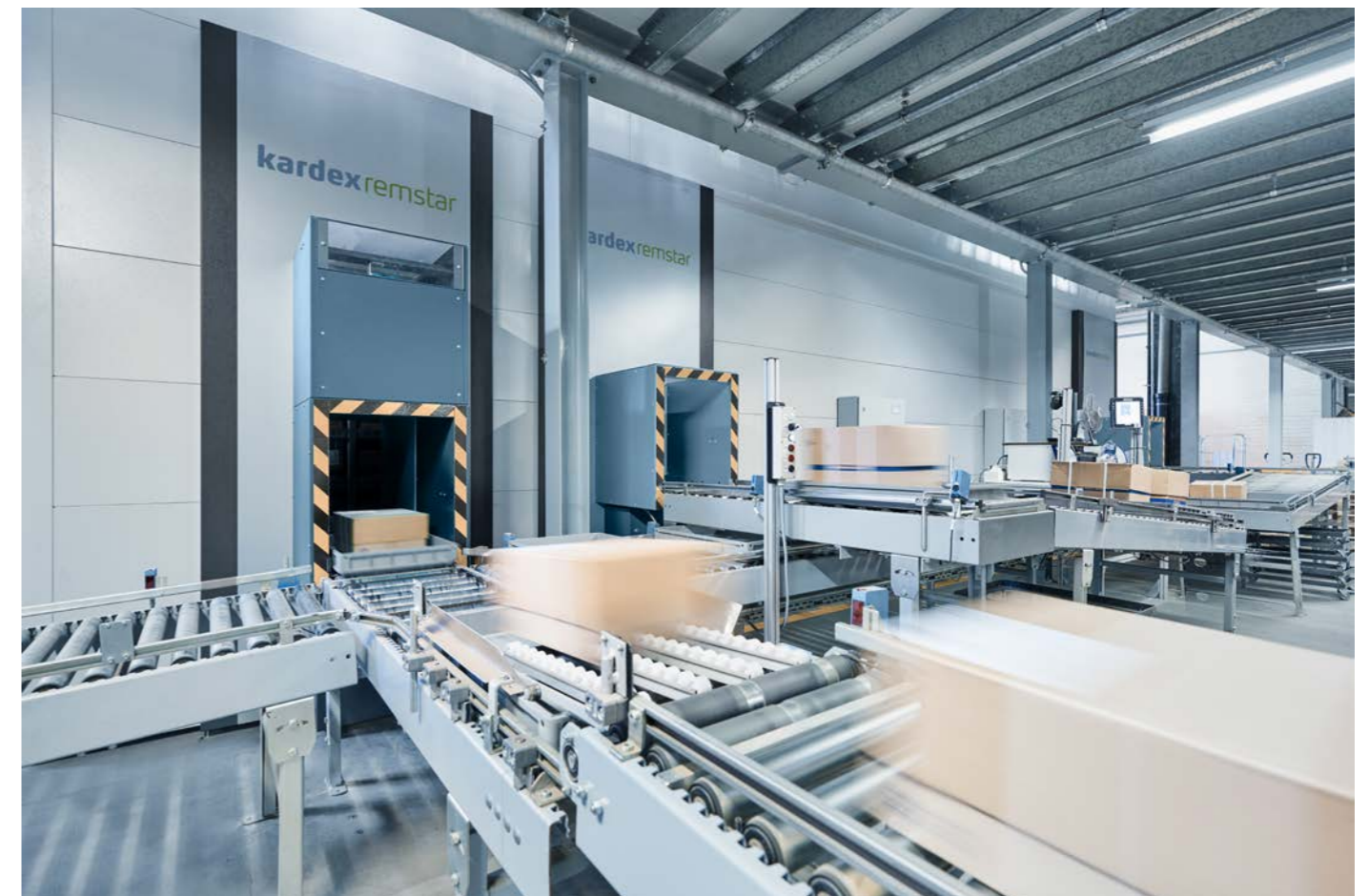
A more advanced order consolidation setup with conveyor bands automatically handling bin distribution.
