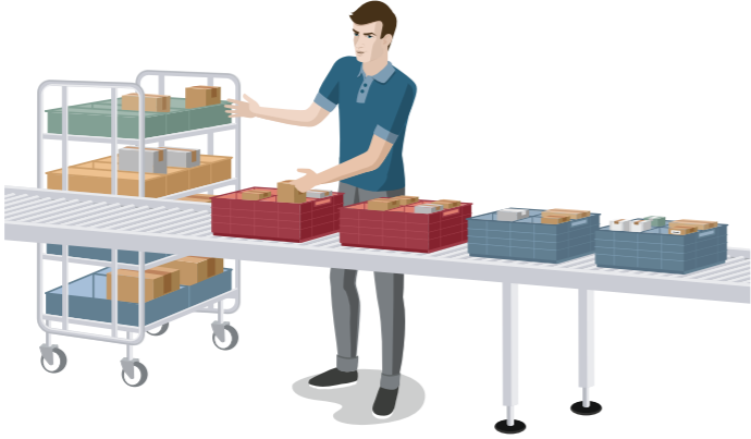
1 Packing of items picked from different zones into boxes (all boxes of the same color correspond to one customer order)
