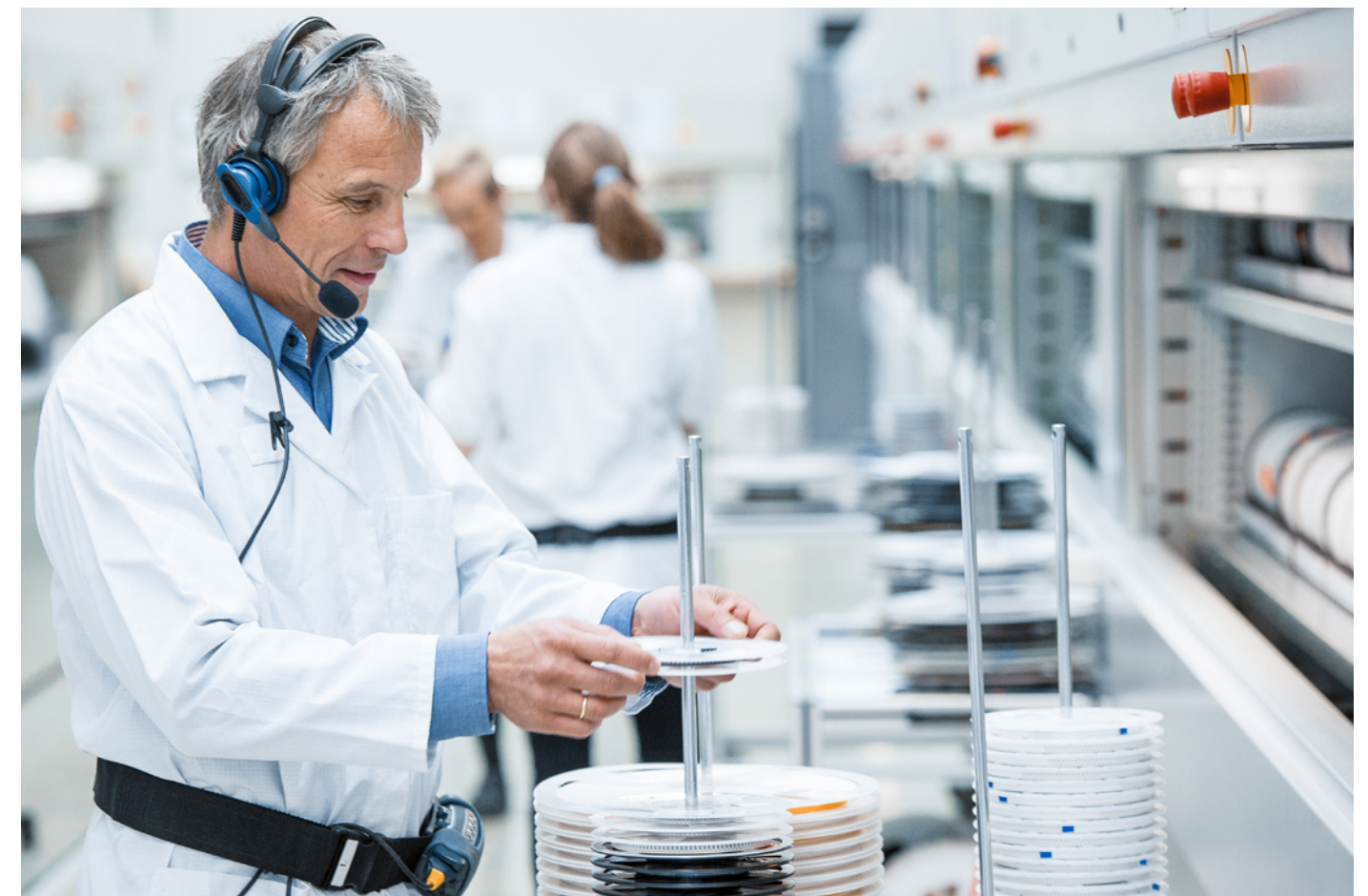
SMD handling with Kardex Megamats
