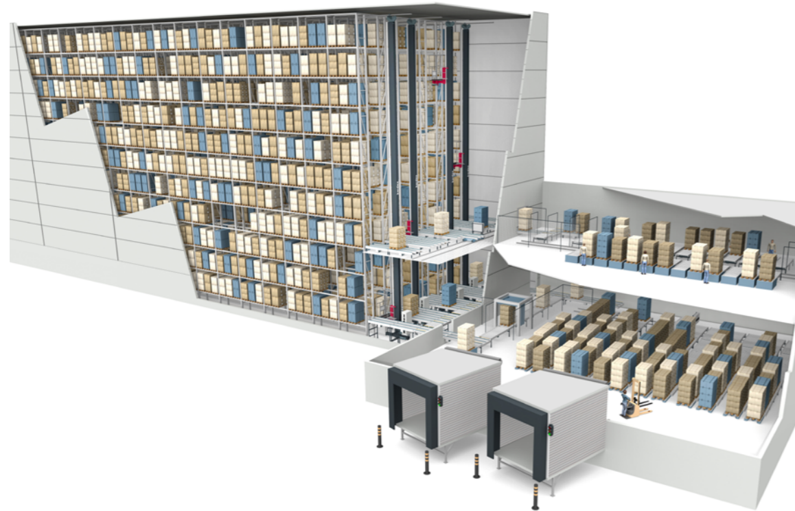
Automated deep-freeze warehouse
