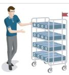
Several picking trolleys with compartments to put the picked items for various customer orders (batches) are used.
