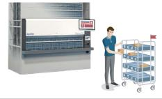
The respective ASRS provides the requested articles and indicates how many to pick and put into which compartment (order) in the trolley.
