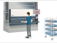
The system assigns a color to each picking trolley. All ASRS with items for this trolley show the corresponding color.
