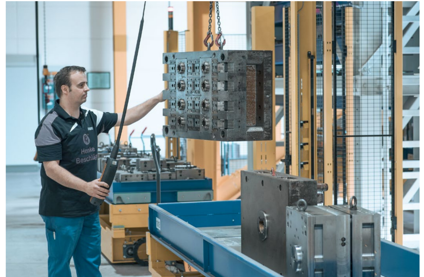
Safe loading / unloading of tools and moulds using by overhead crane
