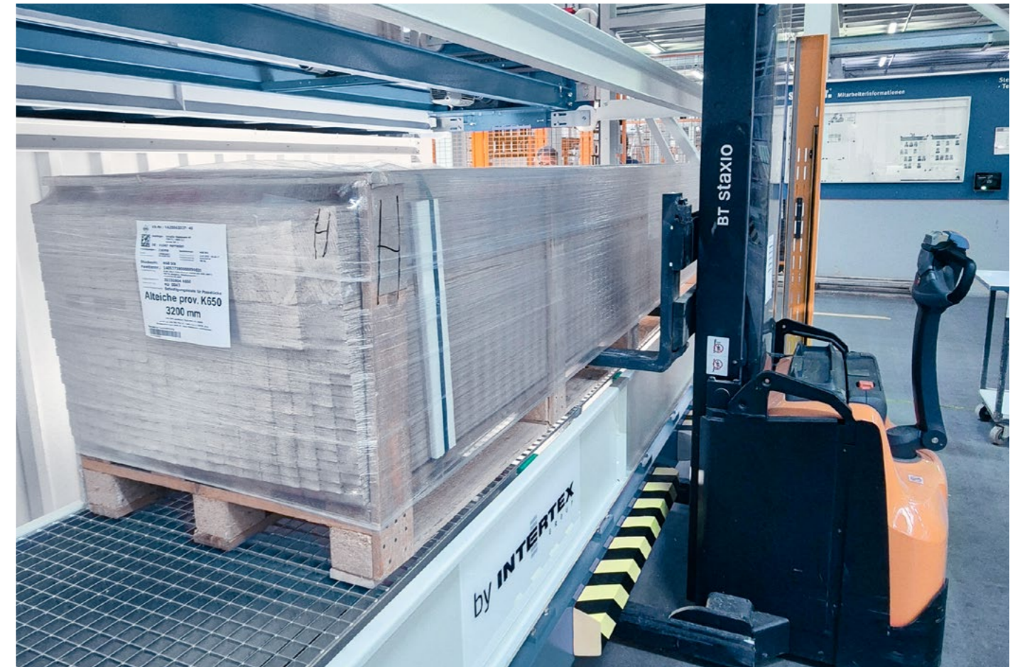
The double bottom in the tray allows pallets with various dimensions to be stored
