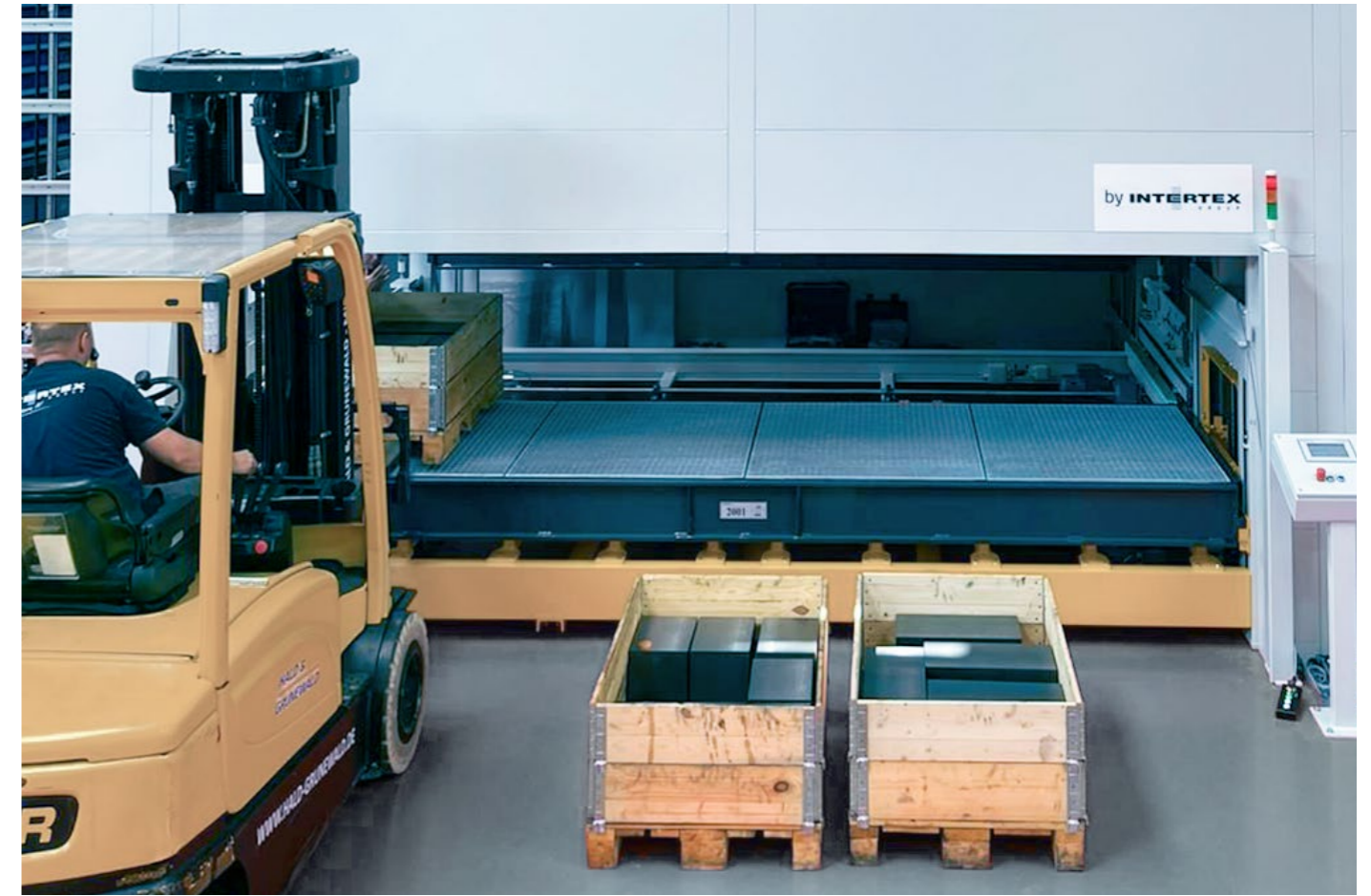
Storage of several Euro-Pallets side by side with a tray width from 3,5m to 8,0m
