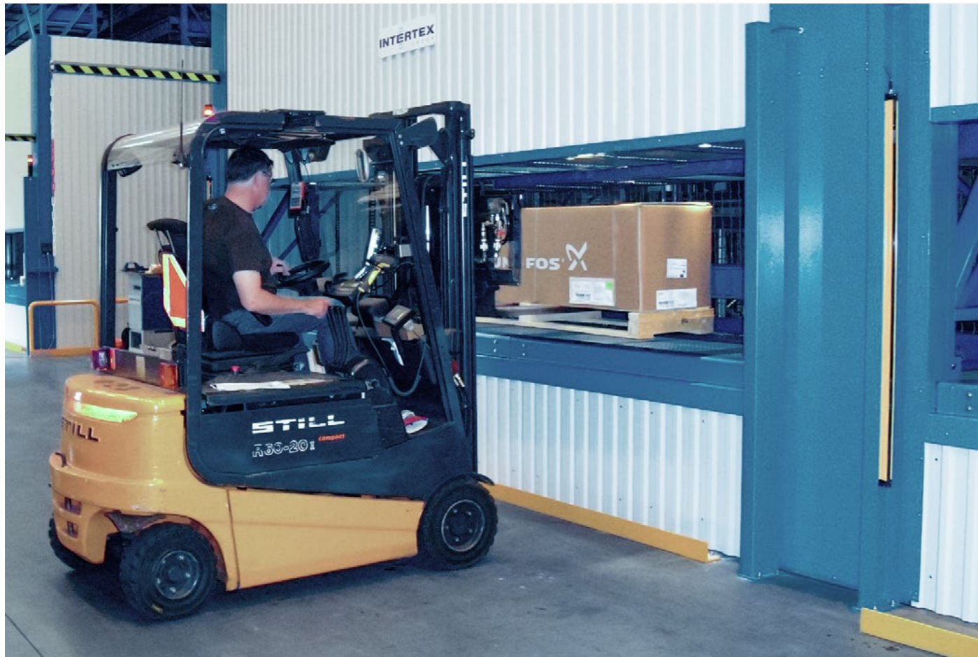
Pallets can be easily stored and retrieved by using the integrated lift/sink station
