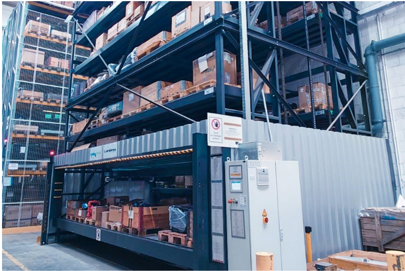
Full utilisation of tray space through the payload of 5,000 kg
