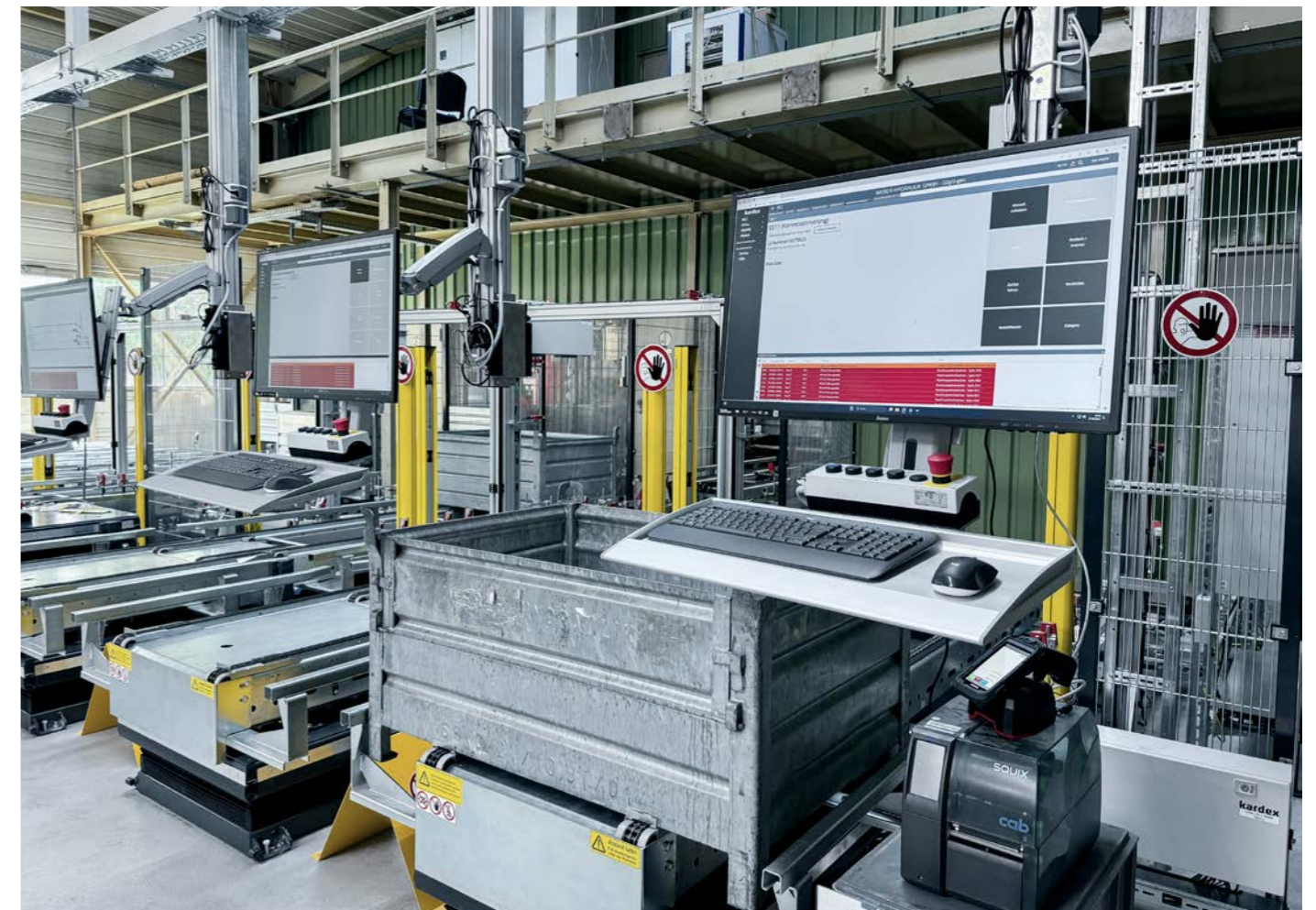
Picking before and after. Improvements were also made in the picking area: This now takes place at five ergonomic, height-adjustable workstations.
