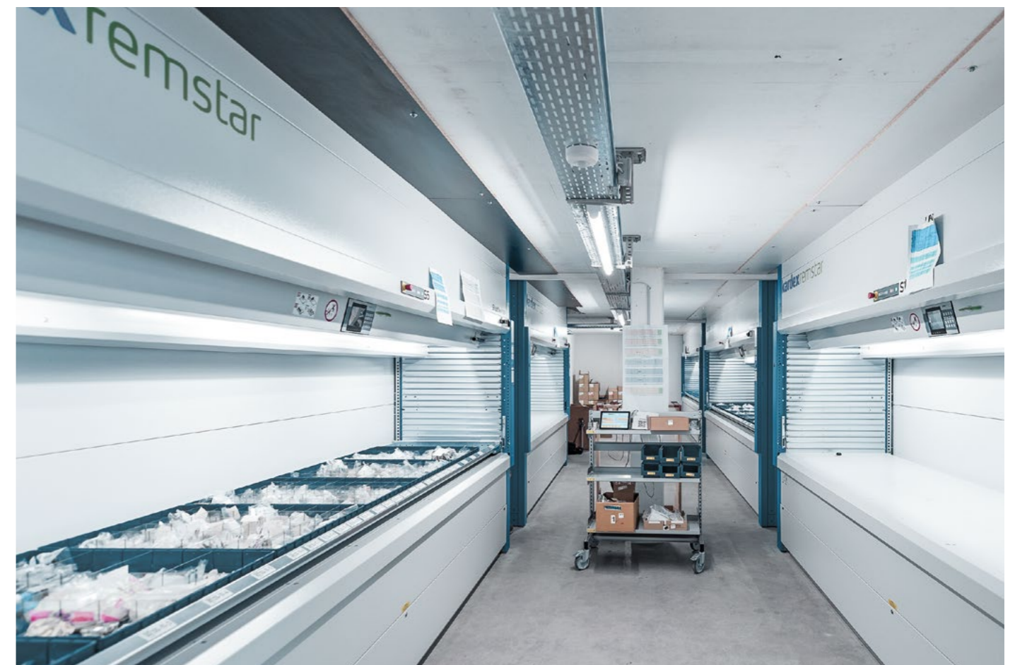
Vertical Lift Module
