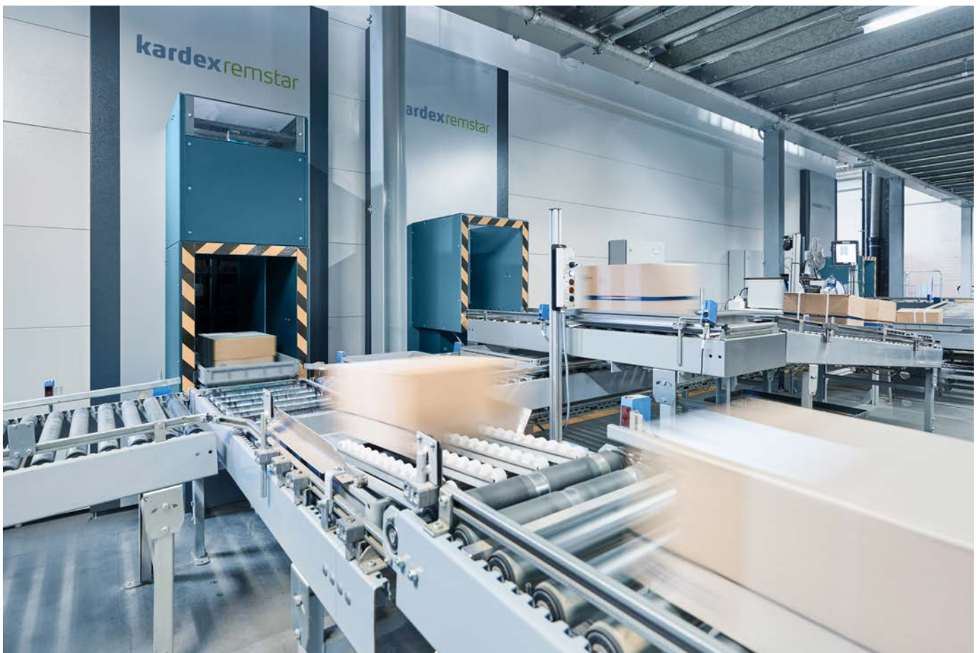
Order consolidation with automatic conveyor connection
