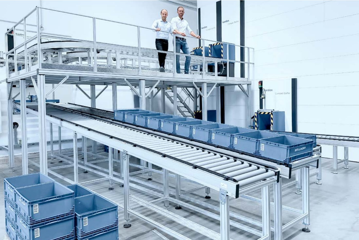
Automated solution with two Kardex Miniload-in-a-Box and conveyor connection
