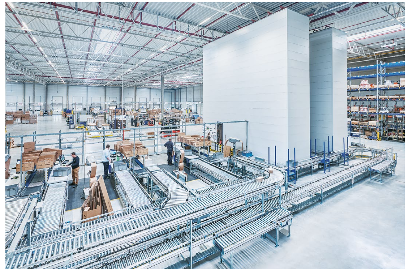
Vertical Buffer Module Kardex Miniload-in-a-Box* with automated conveyor connection
