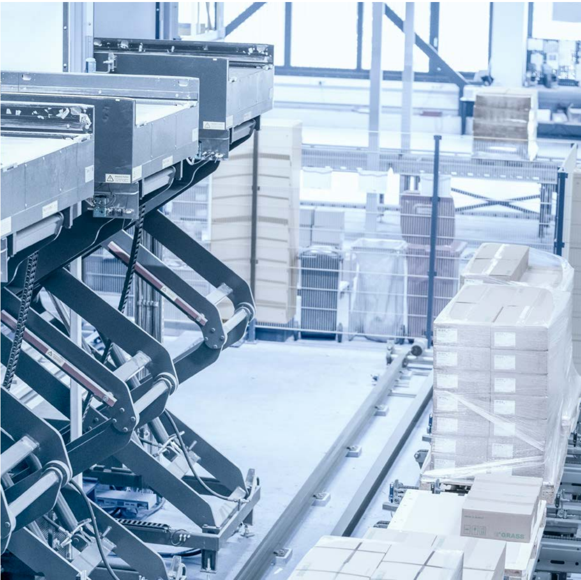
The picking stations are located on a platform that is supplied with the source pallets from the ground floor via eight scissor lift tables.
