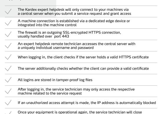
Kardex Connect offers a TÜV-IT certified, HTTPS-connected solution that is more secure and provides more functionality than a VPN or conventional screensharing technologies.
