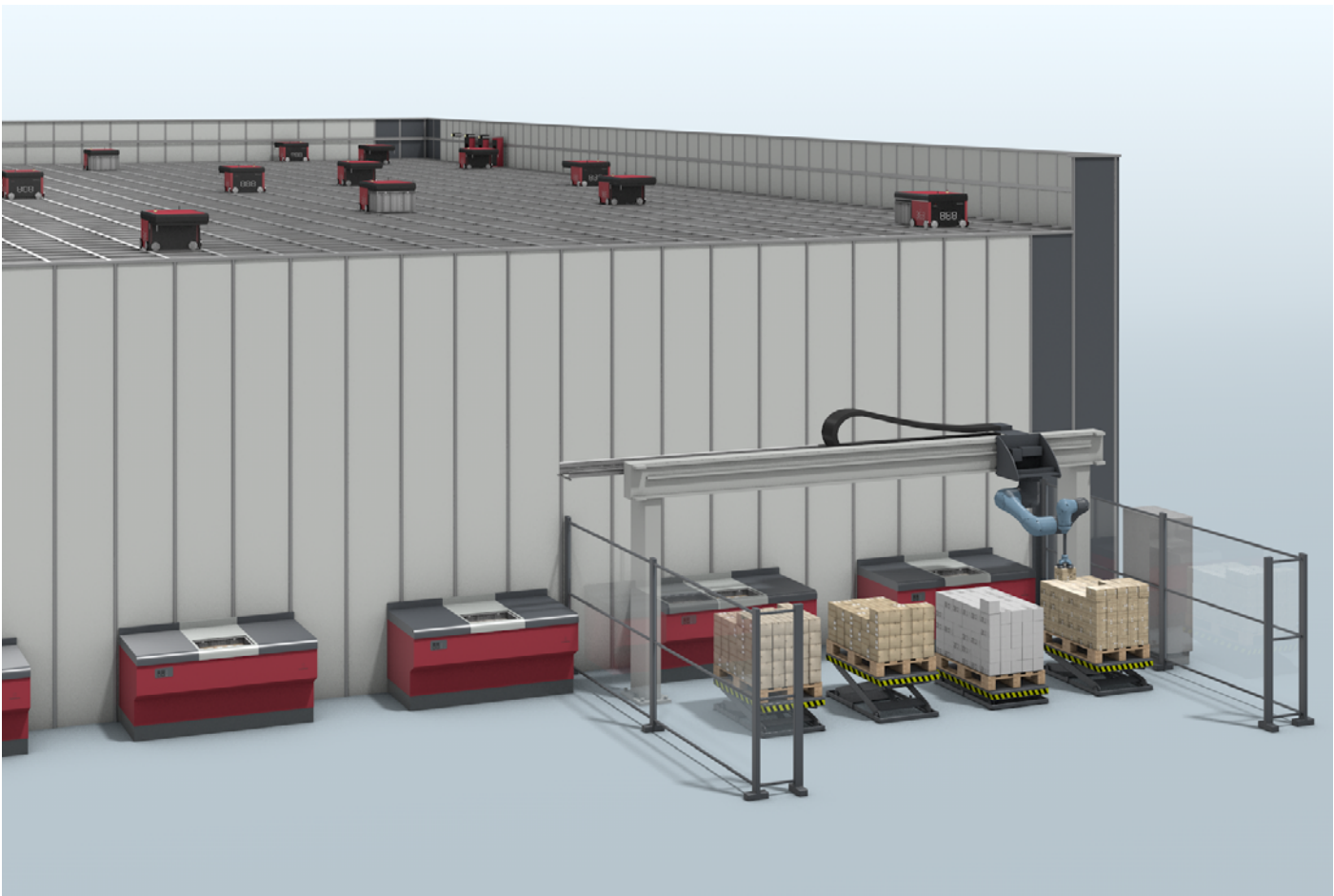
Automated solution with pick and place robotics for (de-)palletizing
