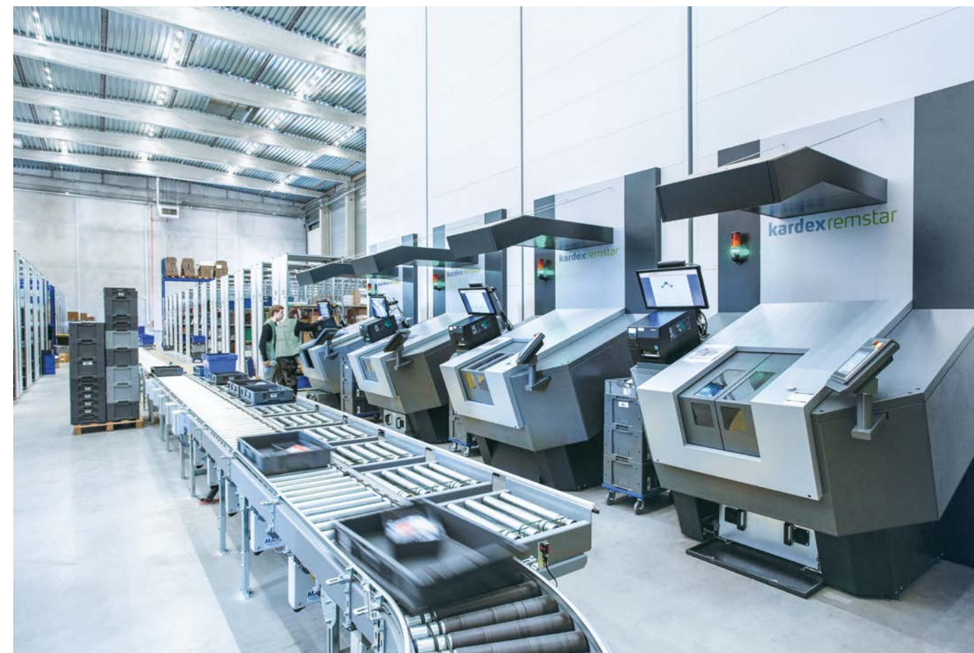
Order picking with turntables and a conveyor system with put locations
