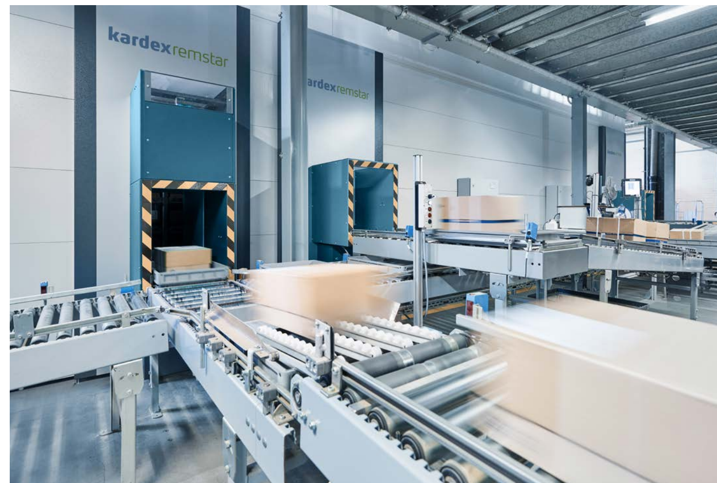
Order consolidation with automatic conveyor connection
