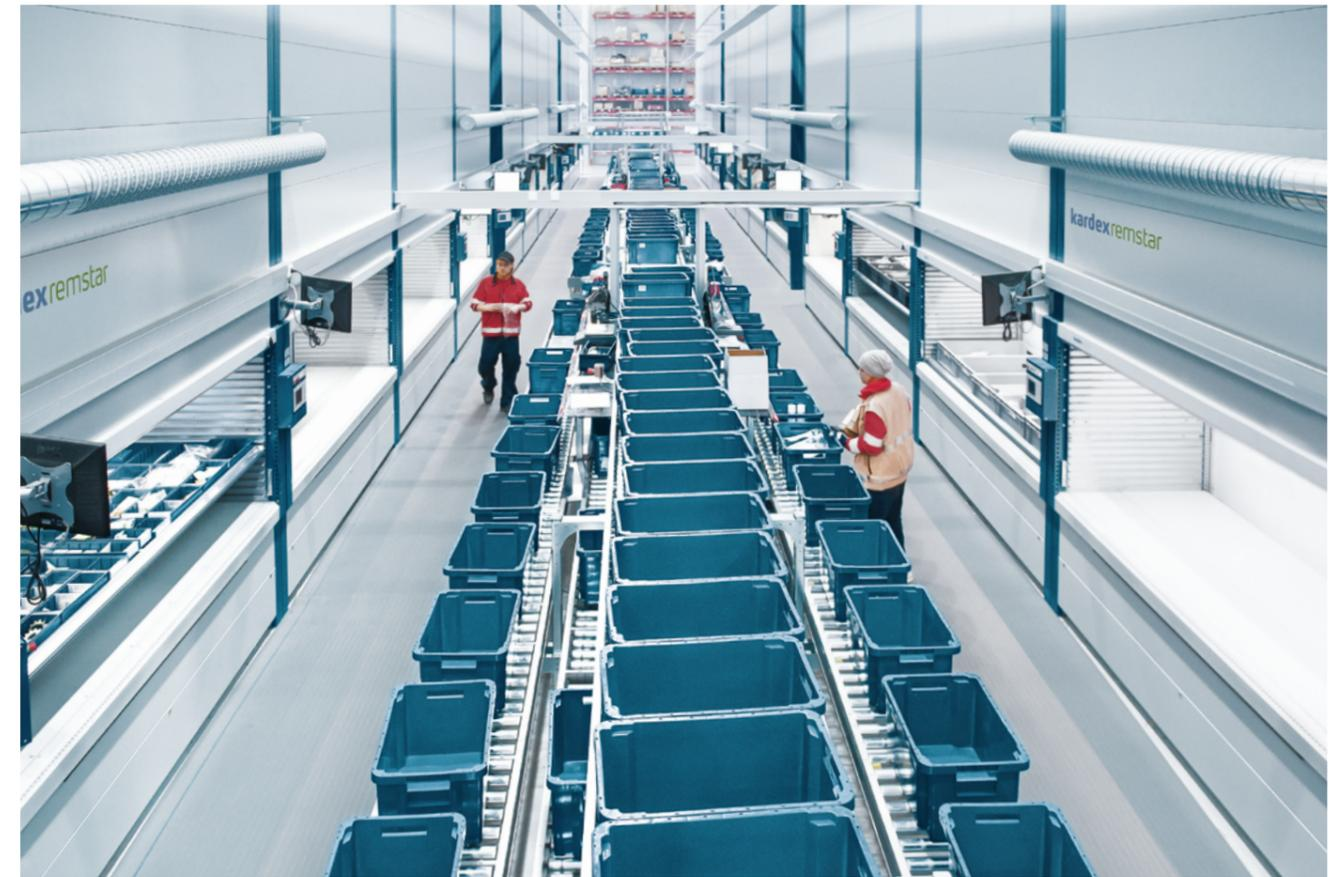
Vertical Lift Module Kardex Shuttle
