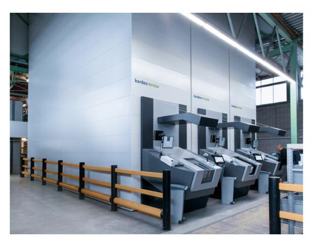
A <u>Vertical Buffer Module (VBM)</u> contains an aisle in the middle of a multi-segment shelving system, where a moveable mast with a telescopic gripper operates. The unit controller sets the gripper in motion picking up a discrete bin/tote and transporting it to a picking station.
