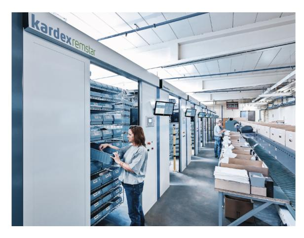
A <u>Horizontal Carousel Module (HCM)</u> consists of an oval track supporting rotating bins with shelves. A motor located inside of the oval track powers the carriers around the track horizontally, stopping at a pre-determined access point for storage or retrieval of goods.
