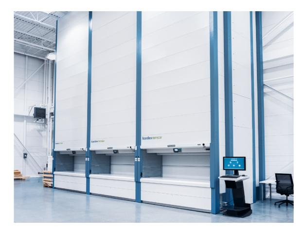
A <u>Vertical Lift Module (VLM)</u> consists of two columns of trays with an automated inserter/extractor positioned in the center. The inserter/extractor travels up and down between the stored trays, automatically locating and retrieving them as needed – similar to an elevator with doors which open on both the front and the rear.
