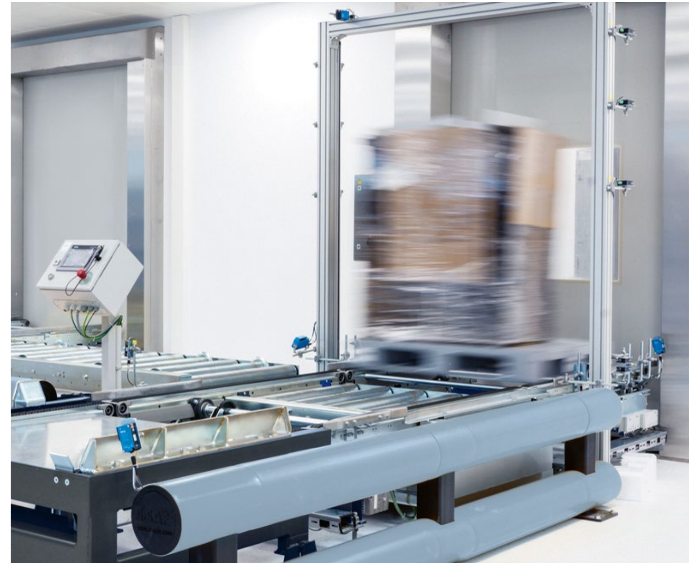
Integrated high-speed doors keep the clean rooms safe and clean and separate them from the grey and black zones.
