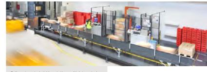
Fully-automated picking stations with integrated lifting platform for ergonomic working.
