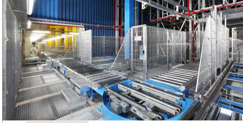
The existing warehouse (at rear) and the new one (in the foreground) were connected by means of the newly installed conveyor systems and integrated in the overall material flow control system.
