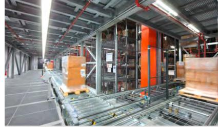
Goods issue/pallet removal with integrated fully-automated labelling machines. Vertical transferunit for 2 pallets, which are picked up together and delivered to the left and right.
