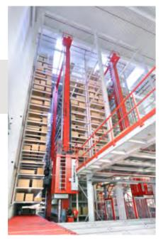
front of the cabinets and by the work surface, which usually dominates the optical appearance. An extremely wide variety of panels is therefore distributed between more than 1,200 storage locations at the Verl-Kaunitz plant, in stacks weighing up to 3.5 tonnes – as much as a small truck. Before the expansion, these panels, as well as the so-called half-format panels and alcove panels, had to be pre-picked at the main plant and transported to the Kaunitz pro-
