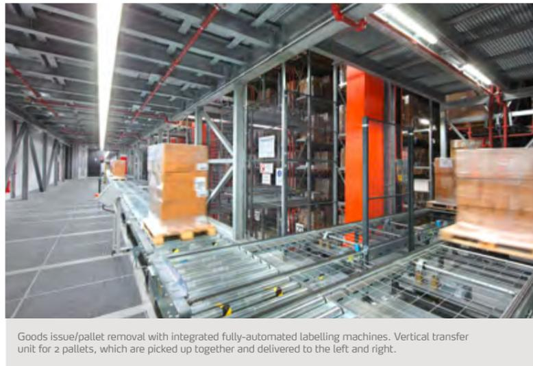
Goods issue/pallet removal with integrated fully-automated labelling machines. Vertical transfer unit for 2 pallets, which are picked up together and delivered to the left and right.
