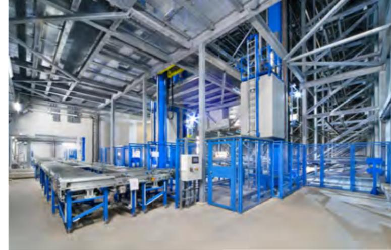
The storage and retrieval level after expansion with a vertical conveyor.
