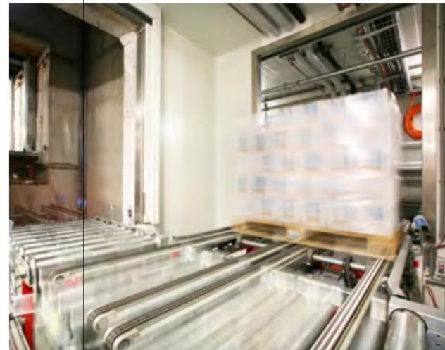
Lifting platforms overcome the differences in level between the individual storage areas, in this case in the passage between the new building and the old one (on the right).
