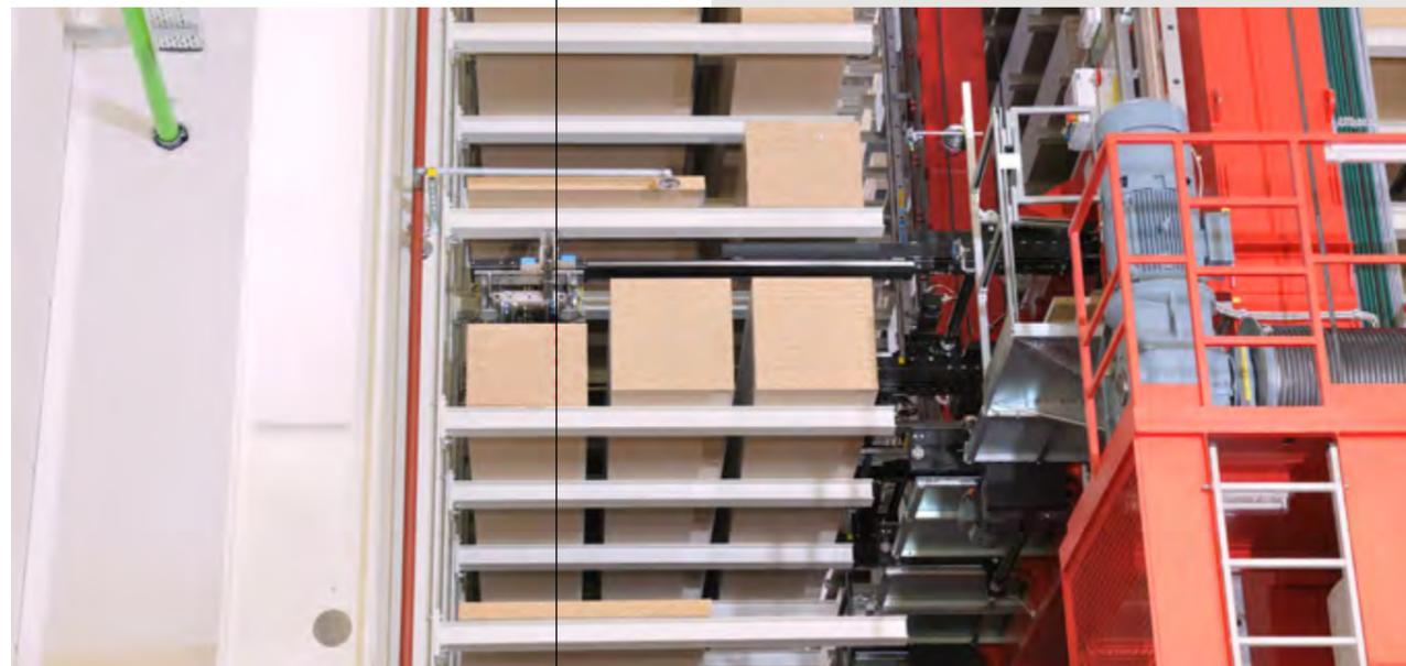
Both S/R machines are equipped with load-handling attachments for triple deep storage. The loads are picked up by two cross-beam vacuum lifters which allow the panels to be separated cleanly from the stacks below.
