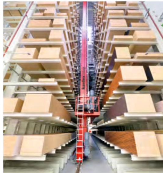
The high-quality individual components of the nobilia kitchens are stored in six zones and on 19 levels. The MTwins serves more than 1,200 storage locations in which a wide variety of different panels are stored in stacks weighing up to 3.5 tonnes.
