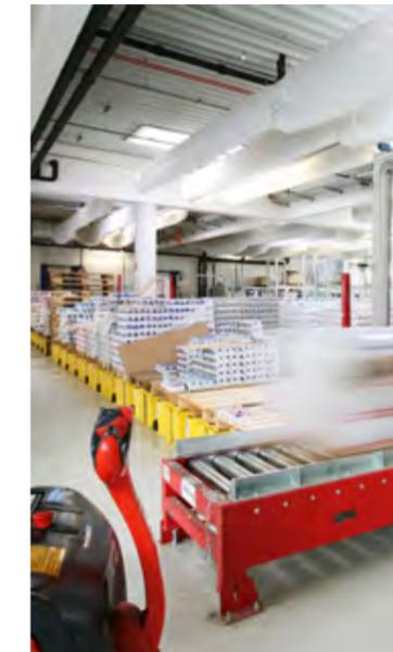
In total, the system as a whole moves between 60 pallets per hour in the picking area, 90 pallets per hour for the removal from storage of the finished products and around 110 pallets per hour on the lower ground floor level. This high performance is not an end in itself, but is of the essence when it comes to the processing of fresh products – after all, once the milk arrives in the shops it should still have the longest possible shelf life.
