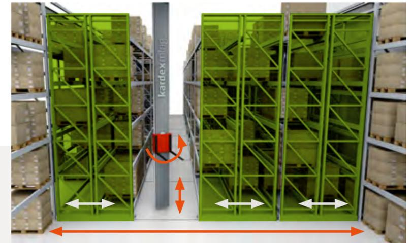
The mobile racking forms an aisle along which the pallet lifting device can access the various pallet spaces
