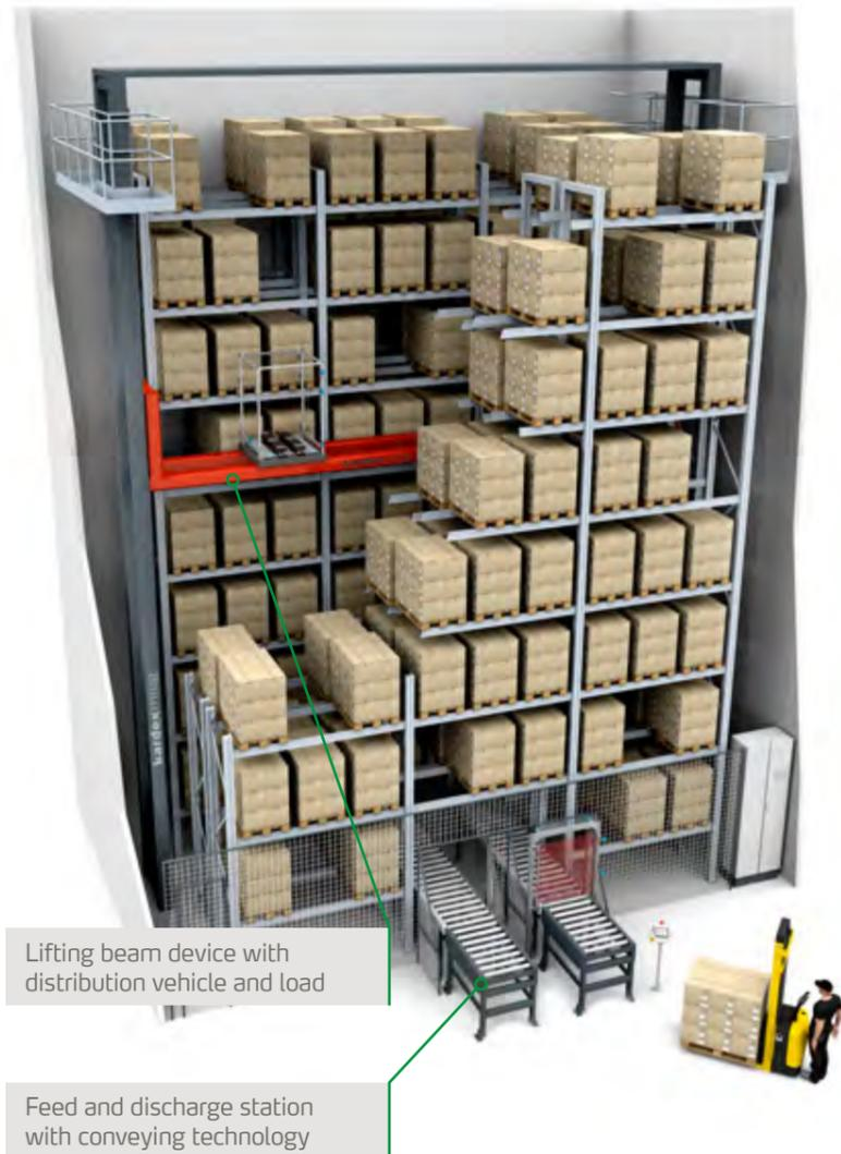
Lifting beam device with distribution vehicle and load
