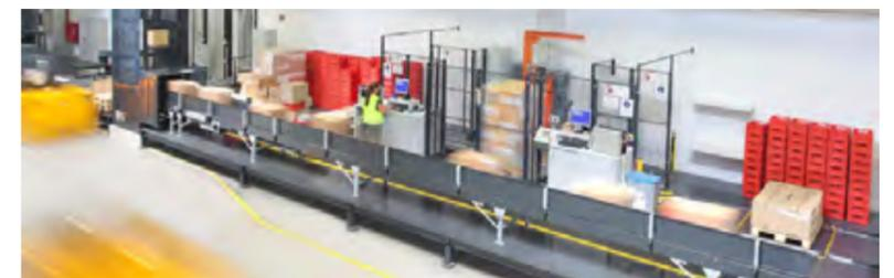
Fully-automated picking stations with integrated lifting platform for ergonomic working.
