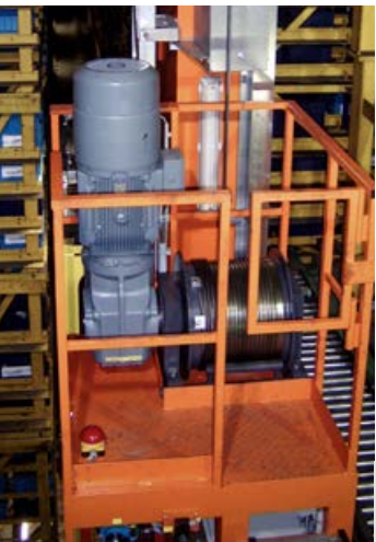
Lift unit of storage and retrieval machine old/new.
