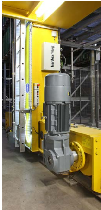
Frequency-controlled chassis motor of storage and retrieval machine.
