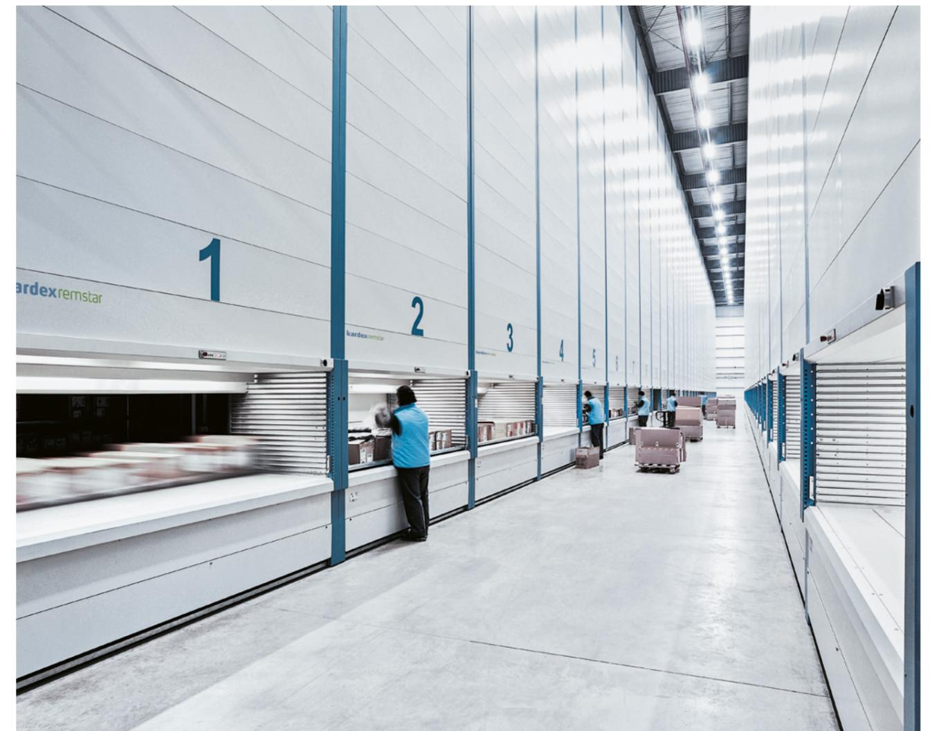
Vertical Lift Module Kardex Shuttle
