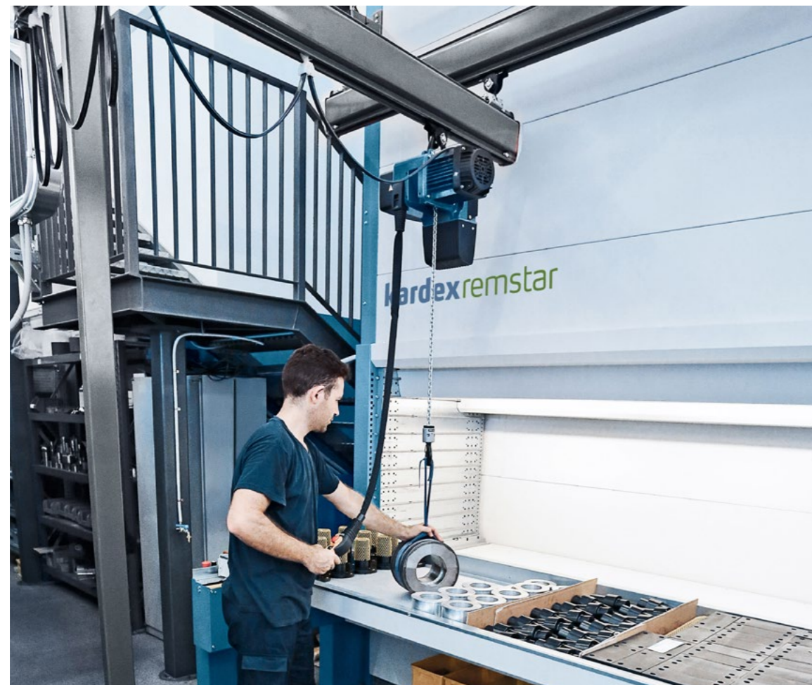
Vertical Lift System Shuttle XP with integrated hoisting crane
