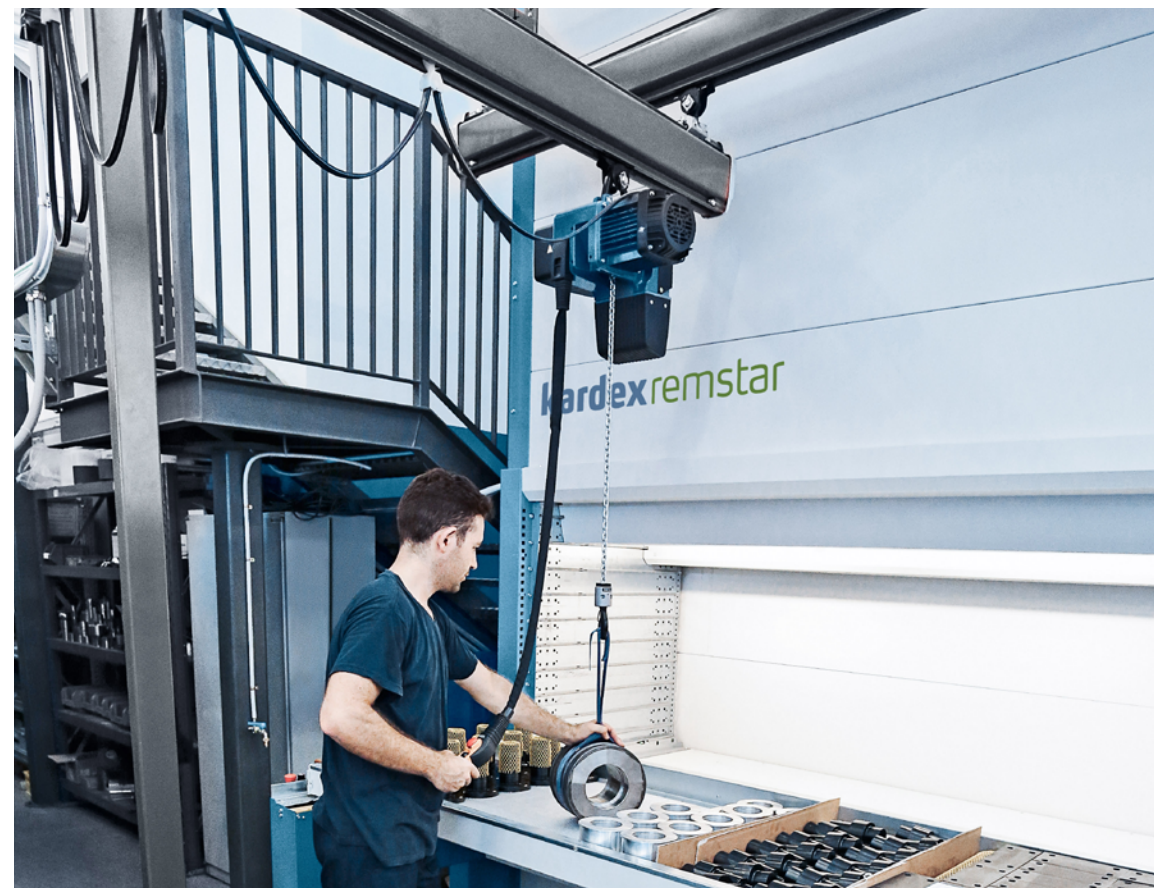
Vertical Lift System Kardex Shuttle with integrated hoisting crane
