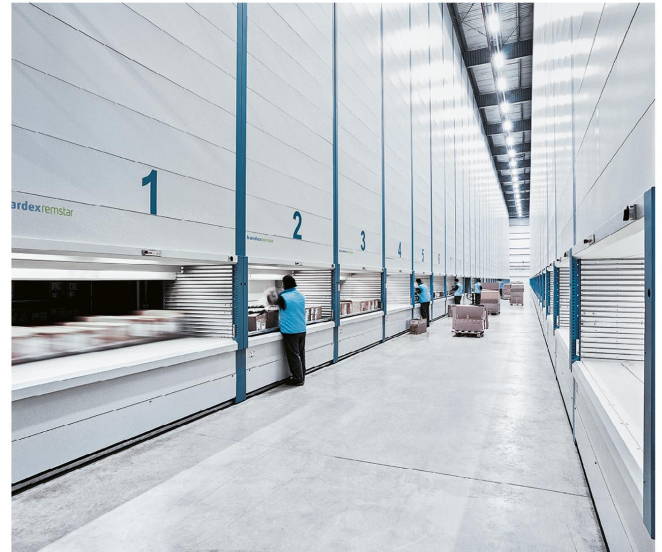
Vertical Lift Module Kardex Shuttle
