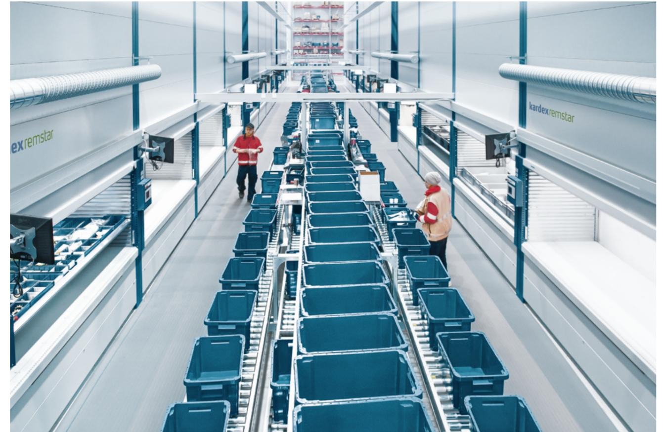
Vertical Lift Module Kardex Shuttle
